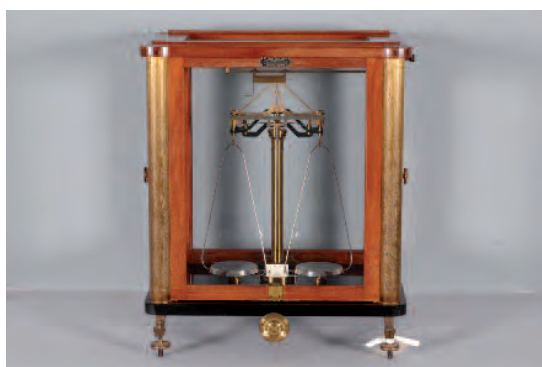
Figure 3. Balance made by F. Sartorius company, Gottingen, Germany (~1908). Catalogue no. 7, School of Chemistry Collection, University of Melbourne. Image credit: Petronella Nel.
