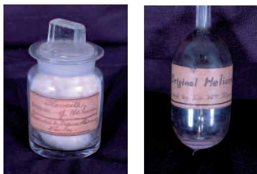
Figure 2. Cleveite sample and helium in a discharge tube (presented by Sir William Ramsay). Cat. nos 155a & b, School of Chemistry Collection, University of Melbourne. Image credit: Petronella Nel.
