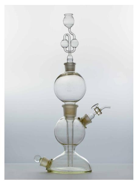
HCl reaches the FeS, hydrogen sulphide gas (H<sub>2</sub>S) is formed and rises to fill the middle chamber. The H<sub>2</sub>S is under slight pressure from the column of HCl. Opening the tap in the middle chamber to draw off H<sub>2</sub>S allows more acid to descend and generate further H<sub>2</sub>S as required. The double bubbler at the very top of the apparatus minimises release into the atmosphere of any H<sub>2</sub>S dissolved in the HCl.
